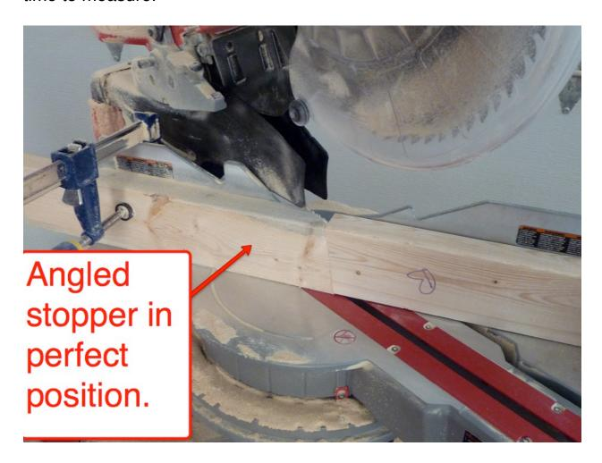
Using this technique you'll be able to quickly pump out perfect looking arrow head cuts like in the pictures below. Check the first few cuts to make sure they're perfect using the **center marker**, if there are some flaws you can correct by re-adjusting the stopper by even just 1/32 of an inch.
