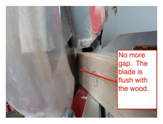
Notice how there is no more gap, the angle of the blade matches the angle of the wood base angle and is perfectly flush with the blade.
