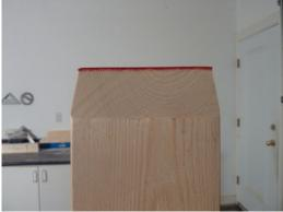
The **center marker** piece is simply a piece with two 45 degree angles cut at exactly the same position on each side of the piece of 2x4. This makes the tip of the "arrow-head" exactly at the center of the wood.
