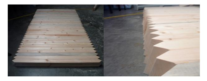
This is the final step, cutting the joint angles, or as I call them the "arrow-head" angles.
