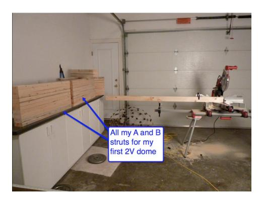
Another critical note on accuracy: When cutting the wood, you want to make sure to always be cutting with the edge of the blade.
