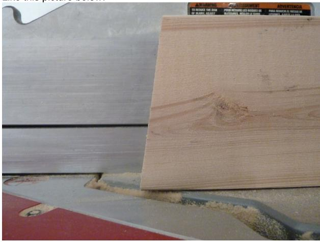
In the case of our dome example, with the 2V dome you'd be angling all the A struts to 15.9 Degrees, and all the B struts to 18.0 Degrees.
