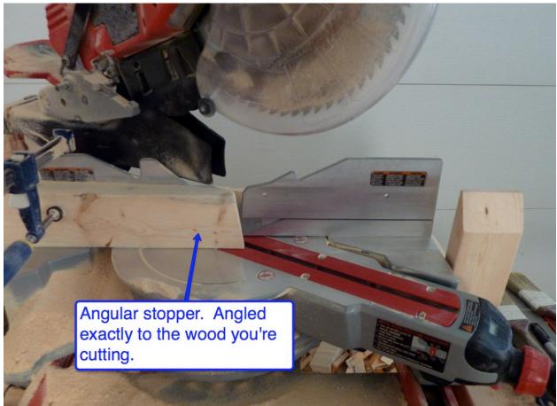
It's just a piece of 2x4 with the same mirror angle that your base angle is. So if you're cutting the A struts in this example, you'd use a scrap piece of wood and angle it at 15.9 degrees and make that your stopper. If it's the B strut, then make a 18 degree stopper:
