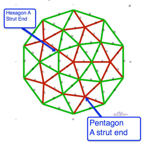
The Geodesic Dome consists of all the struts connected in hexagon and pentagon connections.
